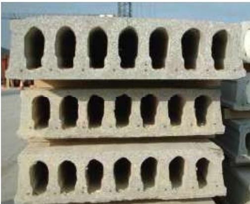
**Figure 17.** Standardised hollow core slabs in widths of 1200 mm generally (also 400, 600, 2400) and depths from 150 to 500 mm in 50 mm increments.
