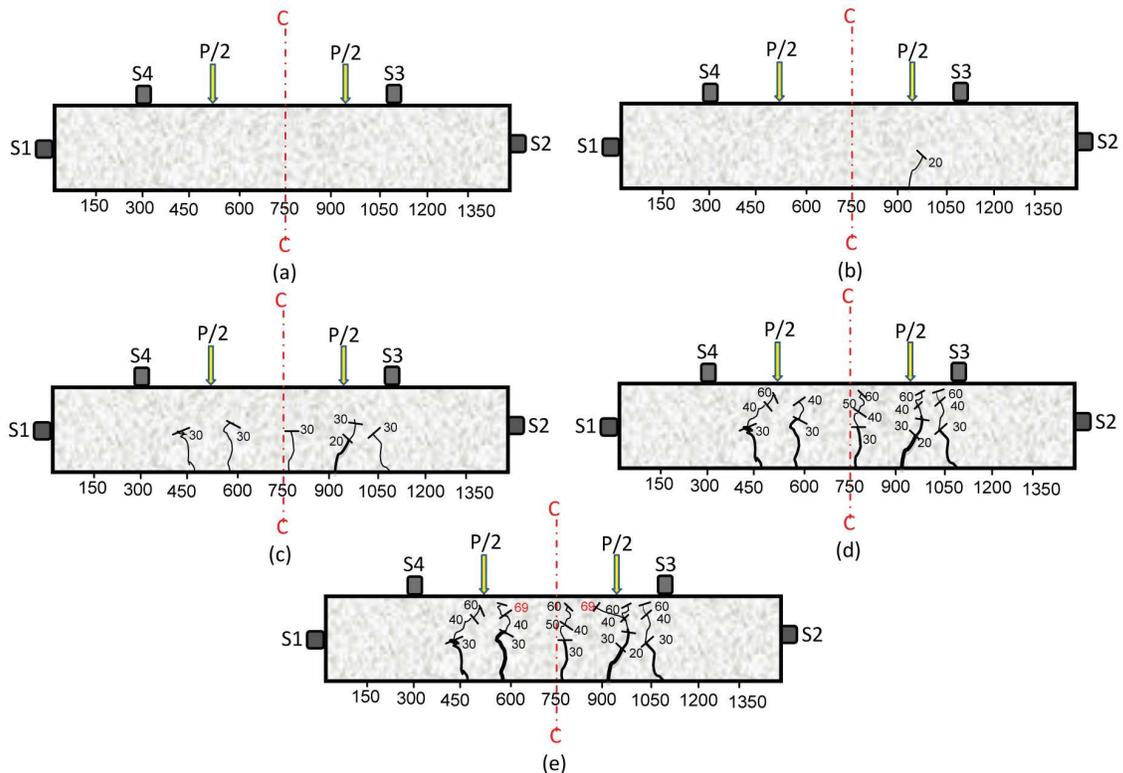
**Figure 6.** Crack patterns obtained by visual observation of all Category I: (a) Stage I- as a micro-cracking , (b) Stage II- as a first visible cracks, (c) Stage III- as a distributed flexural cracks, (d) Stage IV- as a damage localisation , (e) Failure mode. (Load in kN, and distance in mm)
