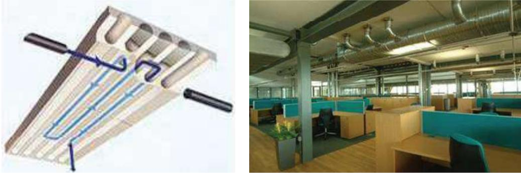
**Figure 24.** Hollow core units with internal labyrinth to circulate the air for ventilation, registered as c. "TermoDeckR"
