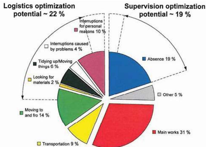
Figure 2. Potential cost reduction of industrialised construction (CIB, 2010)
