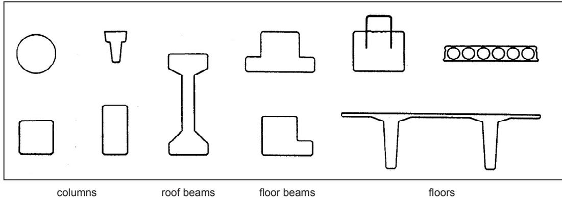
Figure 21. Other examples of standard cross-sections.
