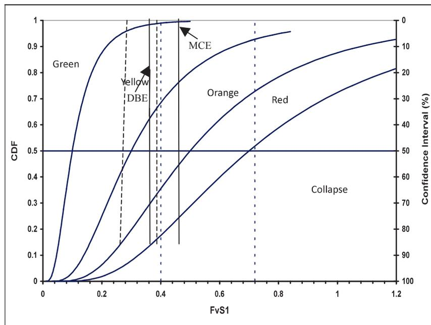
**Figure 4.** Fragility curve for precast double-storey house constructed using shear-key wall panel.
