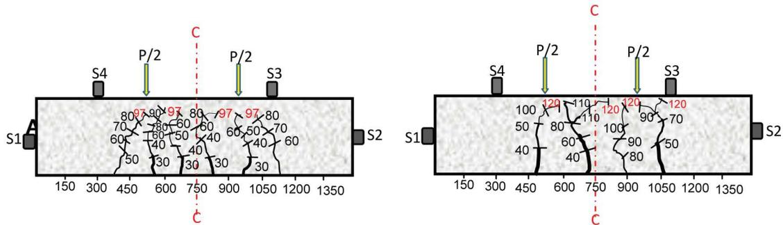
Figure 7. Crack patterns obtained by visual observation at the final stage of damage : (a) TII, (b) TIII. (Load in kN, and distance in mm)
