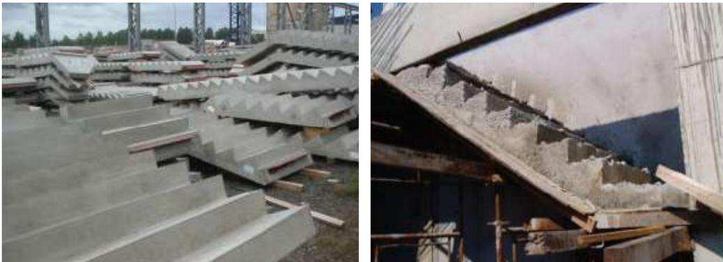
**Figure 15.** The contrasting quality of precast concrete staircases and landings, of ten cast together (left), and cast insitu staircases (right)
