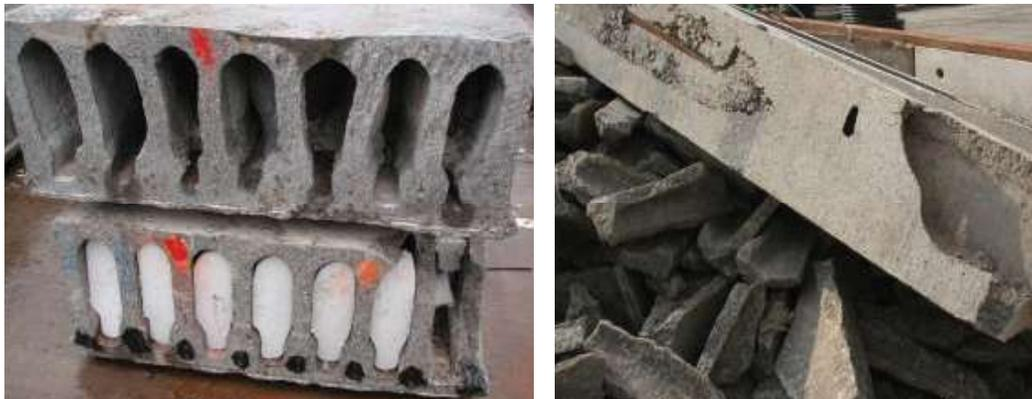
Figure 22. Defective hollow core units are rejected for recycling.
