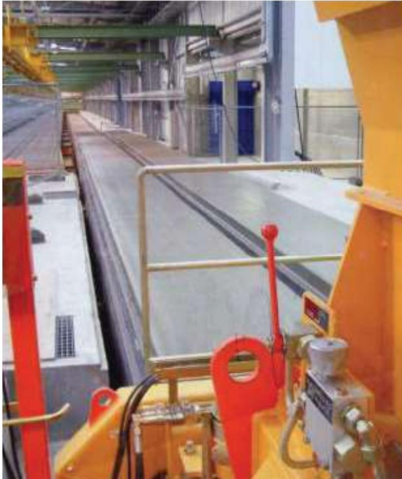
**Figure 5.** Continuous and automated production of prestressed concrete floor slabs by Bison Concrete Products, UK. The slab is made in a continuous length of 180 m, and later cut to length according to project requirements.
