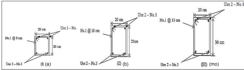
Figure 2. Cross section detailing for beam s: (a) Type I, (b) Type II, and (c) Type III
