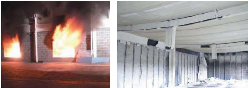
**Figure 12.** Left, three 6.0 m wide bays of 7.0 m span hollow core slabs are on top of the blockwork walls during the 3 hour test which reached 1050°C. Right, afterwards the integrity of the floor was assured. C. Precast Flooring Federation, UK in 2007 (Brown, N. E, 2007)
