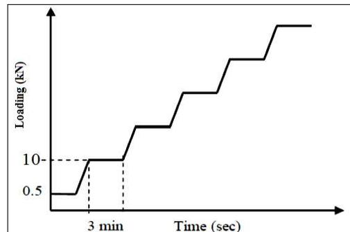
Figure 4. Graphical representation of the stepwise loading
