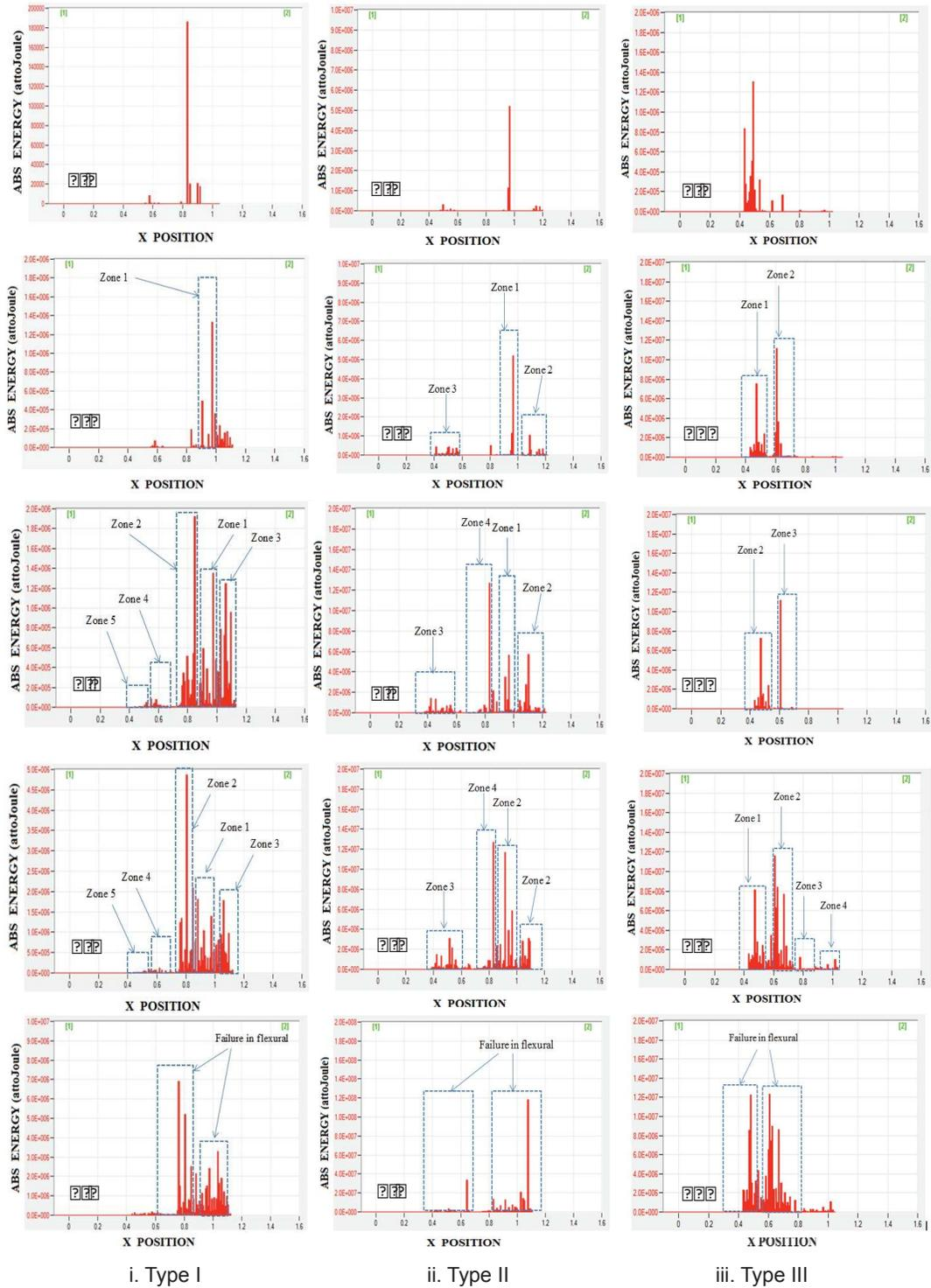
**Figure 8.** AE source location for TI, TII, and TIII: (a) Damage Level I; (b) Damage Level II; (c) Damage Level III; (d) Damage Level IV and (e) Final Failure (from damage level I to failure).
