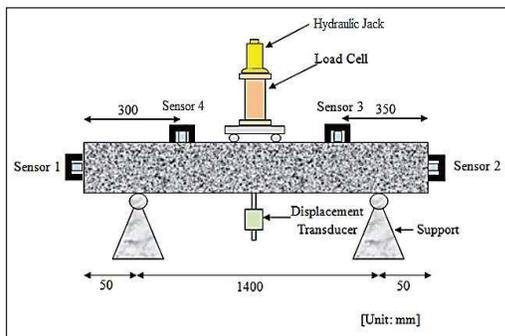
Figure 3. Set up of the four point bending test
