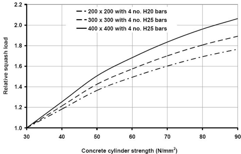
Figure 7. Relative load bearing capacity of columns in relation to concrete strength according to EC2 using high tensile bars grade 500.
