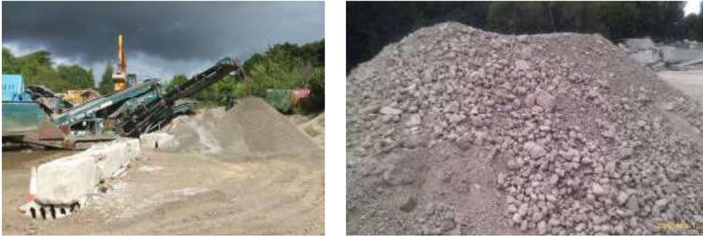
**Figure 23.** (left) Recycling hollow core slabs as RCA, (right) stage 2 processing into sizes.
