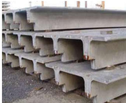
**Figure 18.** Standardised double-tee (or TT) slabs in widths of 2400 mm generally and depths from 300 to 1200 mm in 50 or 100 mm increments, depending on manufacturer.
